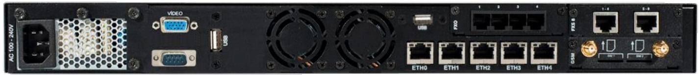
**Legenda:** Vista posterior com 4 FXO (Slot1), 8 FXS (Slot 2) e 2 GSM (Slot 3).
